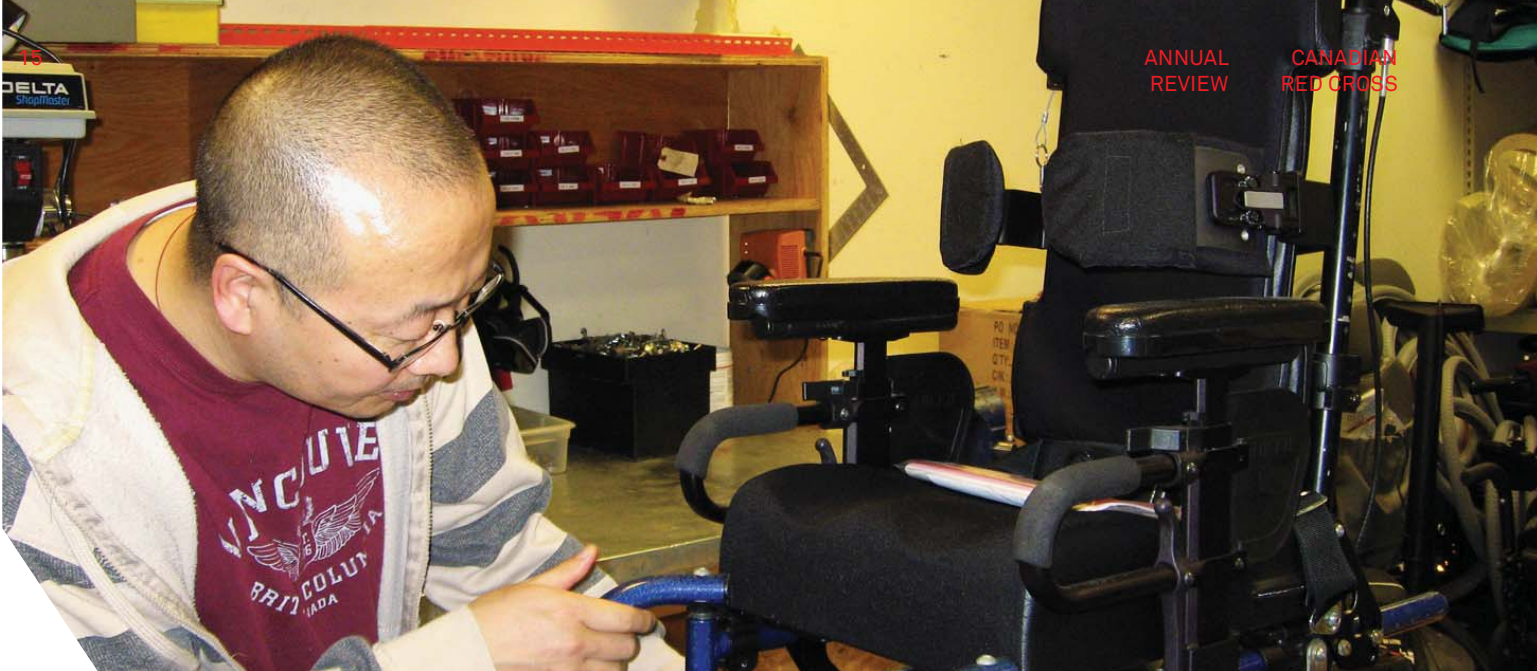
Qing, a technician in the Health Equipment Loan Program workshop, fixing a specialized wheel chair for children.
